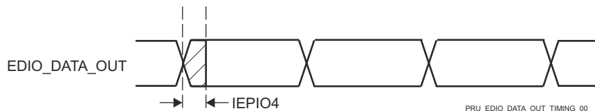
Figure 7-100. PRU_ICSSG IEP Digital IOs Timing Requirements
