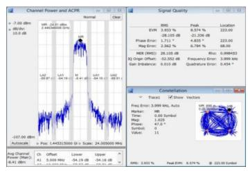
SignalVu-PC application SV26 enables quick, standards-based transmitter health checks on APCO P25 signals. The following image shows a Phase II signal being monitored for anomalies with the spectrum analyzer while performing transmitter power, modulation and frequency measurements.
