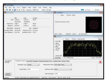
256QAM, (6 MS/s, 2.45 GHz, Root raised cosine filter, -5.00 dBm), RMS EVM: 0.6%
