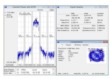
SignalVu-PC Option SV26 enables quick, standards-based transmitter health checks on APCO P25 signals. The following image shows a Phase II signal being monitored for anomalies with the spectrum analyzer while performing transmitter power, modulation and frequency measurements.
