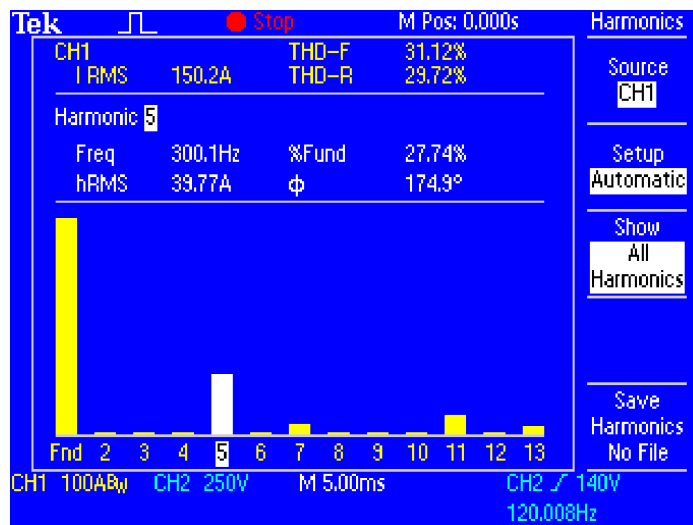
Conduct harmonic distortion measurements with TPS2PWR1 software.
