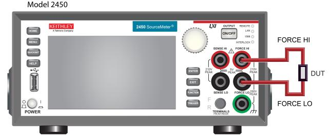
Figure 59: Model 2450 2-wire rear-panel connections
