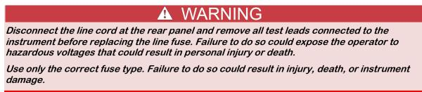
Use a 5 x 20 mm slow-blow fuse rated at 250 V at 2 A.
