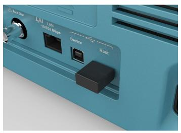
Wi-Fi adapters are configured through integrated setup menus and support seamless wireless communications
