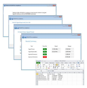
The WLAN presets make the Error Vector Magnitude (EVM), Constellation, and Spectral Emission Mask (SEM) measurements push-button. In addition, you can download the WLAN pre-compliance wizard to easily and quickly prepare for compliance regulatory tests. The Wizard automatically measures Transmit Power, Occupied Bandwidth, Spectral Power Density, Spectral Emission Mask and Spurious Emission Mask.
