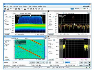
Once captured into memory, SignalVu-PC provides detailed analysis in multiple domains. The spectrogram display (bottom left panel) shows the frequency of an LFM pulse changing over time. By selecting the point in time in the spectrogram during the On time of the pulse, the chirp behavior can be seen as it sweeps from low to high (upper right panel).
