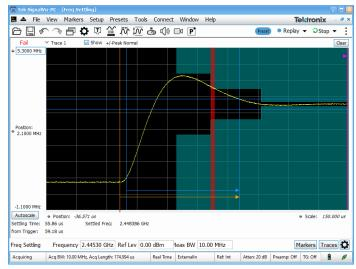
Settling time measurements (SVT) are easy and automated. The user can select measurement bandwidth, tolerance bands, reference frequency (auto or manual), and establish up to 3 tolerance bands vs. time for Pass/ Fail testing. Settling time may be referenced to external or internal trigger, and from the last settled frequency or phase. In the illustration, frequency settling time for a hopped oscillator is measured from an external trigger point from the device under test.
