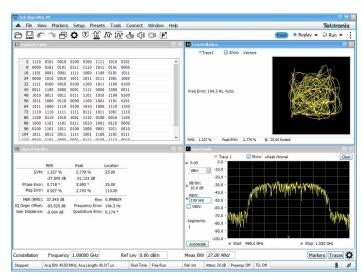
Wideband satellite and point-to-point microwave links can be directly observed with SignalVu-PC analysis software. Here, general purpose Digital Modulation Analysis (SVM) is demodulating a 16QAM backhaul link running at 312.5 MS/s.
