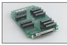
**STA-300:** Screw Terminal Accessory. Mounts on a panel and includes nylon standoffs for tabletop applications. Requires a CAB-305 cable.
