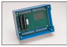
**STA-U:** The STA-U is a universal screw terminal accessory designed to connect to many Keithley data acquisition boards. It includes one 25-pin female D-type connector and two 37-pin male D-type connectors tied together. All 37 lines are brought out to screw terminal connections. A small breadboard area is available for additional circuitry. The STA-U is used for direct connec-
