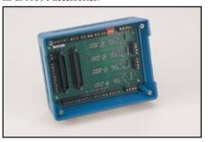
**STA-MB:** The STA-MB Screw Terminal Accessory provides sockets for 4 MB-Series modules. Two parallel 37-pin D male connectors provide interfaces for DAS boards and accessories. The MB-Series module inputs and outputs as well as the I/O connector pins are brought out to screw terminals. You then wire the MB-Series outputs to pins on the I/O connectors according to the requirements of your application.
