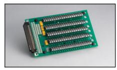
**KUSB-STP100**: Screw terminal panel with 100pin, male, D-type connector. This screw terminal panel will only work with the KUSB-CABDIO. For use with KUSB-3160.
