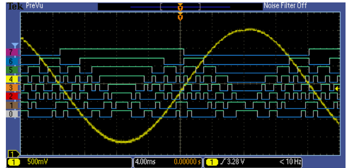
Figure 9: The MSO Series provides 16 integrated digital channels enabling you to view and analyze time-correlated analog and digital signals.
