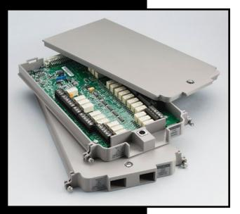
The Model 7751, 7752, and 7753 Source/Switch Modules are designed exclusively for use in the Model 2790 SourceMeter Switch System for electrical checks of airbag inflators and a variety of other automotive electrical test applications. These modules provide the programmable high voltage and low current sourcing, plus the multichannel switching support required to measure insulation resistance and conductor continuity in these applications.
