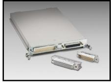
The Model 7707 plug-in module offers 10 channels of 2-pole or 5 channels of 4-pole multiplexer switching that can be configured as two independent banks of multiplexers. The Model 7707 also provides 32 digital input/output channels (four 8-bit ports) for I/O control. Connect the Model 7707 to industry standard solid-state
