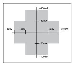
The Model 6430 provides four-quadrant sourcing of up to 2.2W, as well as measurement sensitivity down to sub-femtoamp and microvolt levels. It can measure currents from the 1pA range (with just 0.4fA p-p noise typical) up to the 100mA range at up to 20V. Voltage ranges from 200mV to 200V are available. Current and voltage range settings define the maximum source or sink voltage or current.
