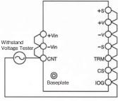
3kVAC 1 minute (20mA) (48VDC Input Model: 1.5kVAC)
