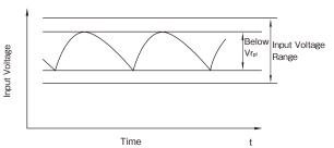
Figure1-2: Input Ripple Voltage
