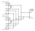
Figure3-1: Parallel Operation
