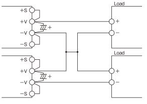
Figure12-2 ±Output Series Operation
