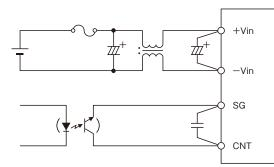
Figure10-1: Connection of CNT Terminal
