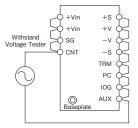
3kVAC for 1 minute (20mA) (24VDC Input model: 2kVAC) Figure21-2: Withstand Voltage Test between Input and output
