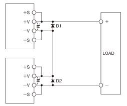
Figure12-1: Series Operation for High Output Voltage Configurations
