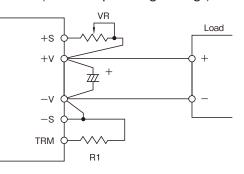
Figure2-7: Connection Example of External Resistor
