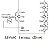
(48VDC Input Model: 1.5kVAC)
