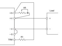
Figure2-2 Example Connection of External Resistance
