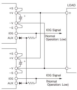
Figure13-1: Example of IOG Terminal Connection
