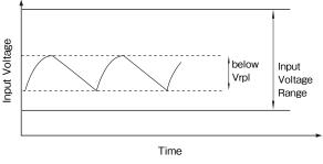
Figure1-1 Ripple Voltage
