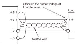
Figure9-1 Remote Sensing at Use
