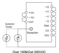
Figure21-1 Isolation Test
