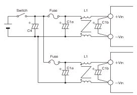
Figure1-5 : Input Filter when several power modules are connected
