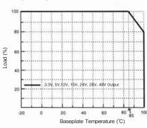
Figure14-1Output Derating Curve
