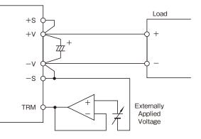
Figure2-9: Example of Applied Voltage
