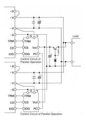
Figure3-5 Example: Vcc is supplied by +V
