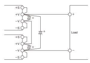
Figure12-1 Series Operation in High Output Voltage
