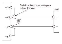
Figure9-2 Remote Sensing Not in Use
