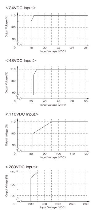
Figure2-1 : Limitation of Input Voltage Range
