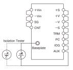
(more than 500M  $\Omega$  between the output and baseplate at 500VDC) Figure22-1: Insulation Test
