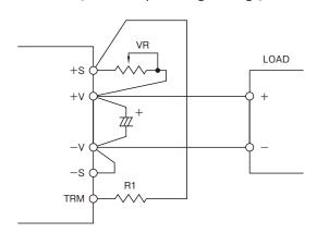
Figure2-4: Connection Example of External Resistor Network #3 PH100S/PH150S
