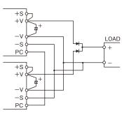
Figure4-1: N+1 Redundant Operation
