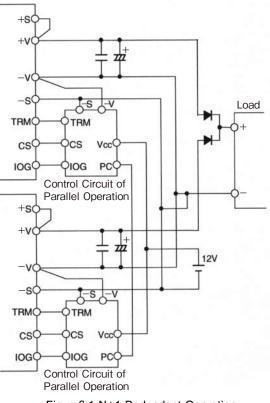
Figure6-1 N+1 Redundant Operation
