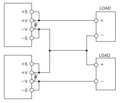
Figure 12-2: Series Operation using  $\pm$  Output
