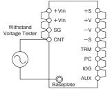
2.5kVAC for 1 minute (20mA) (24VDC Input model: 2kVAC) Figure21-1: Withstand Voltage Test between Input and Baseplate
