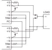
Figure 4-2: N+1 Redundant Operation with programmed output voltage
