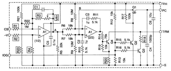
Figure3-2 Control Circuit fo Parallel Operation
