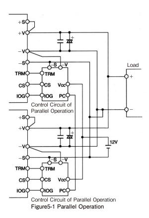
(b) Parallel Operation programmed output voltage
