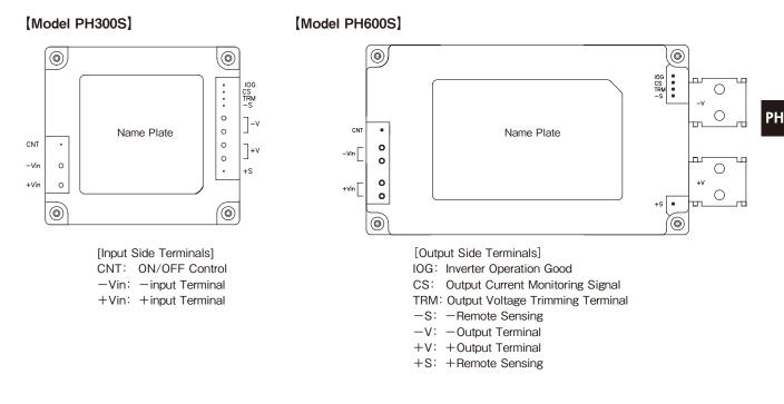
Baseplate can be connected to FG through M3 mounting tapped holes. Connect +Vin, -Vin, +V, -V with consideration of contacting resistance.
