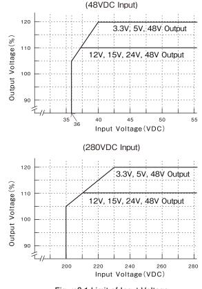
Figure2-1 Limit of Input Voltage
