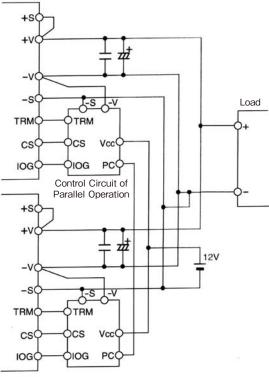
Control Circuit of Parallel Operation
