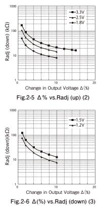
(3) To adjust output voltage for whole range Resistor values, as well as, connecting methods for external resistor (R1) and external variable resistor (VR) are described below.
