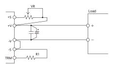
Fig.2-6 Example connection of external resistor
