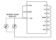
100M Ω and above at 500VDC Fig.20-1 Isolated test
