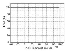
Fig.1-6 Output Derating by PCB Temperature
