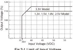
Fig.2-1 Limit of Input Voltage
