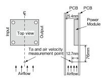
Fig.1-1 Output derating set-up condition
