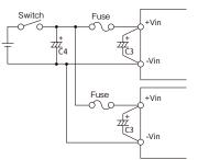
Fig.1-4 Input Filter with Switch when Plural Power
