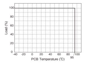
When using with different measurement conditions from output derating by ambient temperature, use output derating by PCB temperature.
