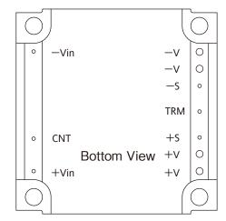
Input and Output Terminal Configurations(Bottom View)
