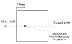
Fig.13-1 Measurement Point of Baseplate Temperature
