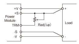
Fig.2-4 Connection for output voltage trim up
