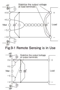
Fig.9-2 Remote Sensing is Not in Use
