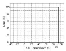
Fig.1-6 Output Derating by PCB Temperature
