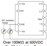
Fig.20-1 Isolation Test
