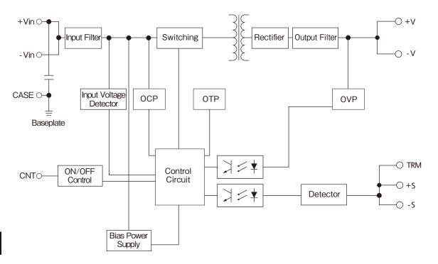
Switching Frequency (fixed) : 400kHz (typ.) for 28V Model, 460kHz (typ.) for 48V Model
