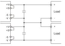
Fig.12-2 Series Operation due to  $\pm$ Output
