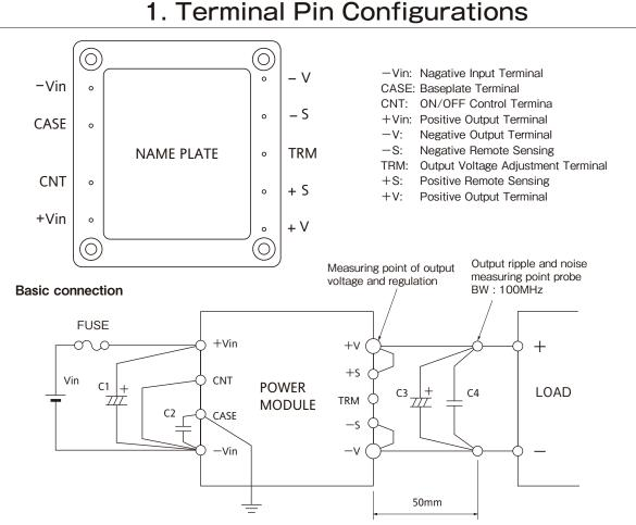
Note : This diagram is for Negative Logic "ON/OFF" Option.
