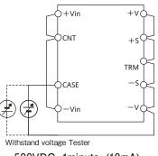
500VDC 1minute (10mA) Fig.19-2 Withstand Voltage Test for Output-Baseplate
