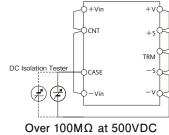
Fig.20-1 Isolation Test
