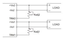
If the external resistor (R<sub>adj</sub>) is connected between the TRIM pin and -Vo pin, the output voltage will increase. Diagram shown below is the output voltage trim up connection.
