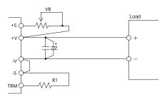
Fig.2-6 Example connection of external resistor
