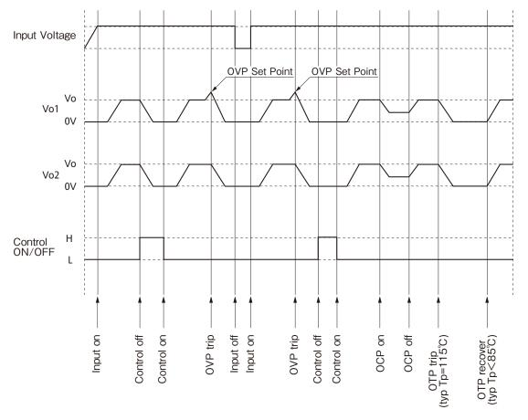
Note: This timing diagram is for Negative Logic "ON/OFF" Option.
