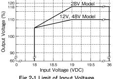
Fig.2-1 Limit of Input Voltage
