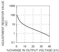
If the external resistor ( $R_{adj}$ ) is connected between the TRM pin and +S pin, the output voltage will increase. Diagram shown below is the output voltage trim up connection.
