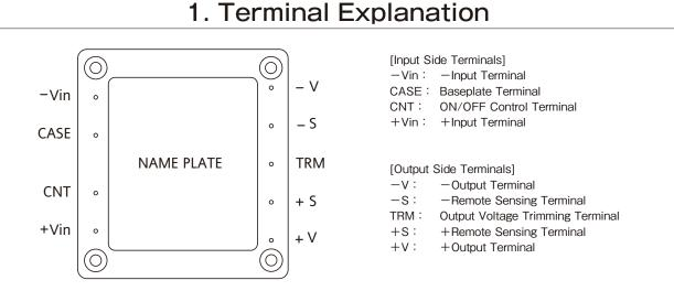
Baseplate can be connected to FG (frame ground) M3 threaded holes (standard model). Connect +Vin, -Vin, +V, -V with consideration of contacting resistance.
