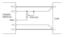
Fig.2-4 Connection for output voltage trim up
