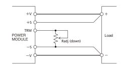
Fig.2-2 Connection for output voltage trim down
