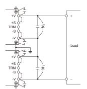
Fig.12-1 Series Operation due to High Output Voltage
