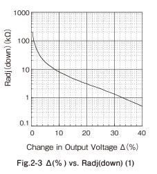
(2) In case of adjusting output voltage higher
