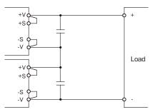
Fig.12-1 Series Operation due to High Output Voltage
