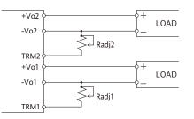
The equations and graphs for the required external resistor ( $R_{adj}$ ) value to obtain a percentage output voltage change of  $\Delta$  Vo% is as shown in the next page.
