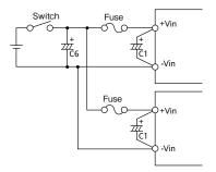
Fig.1-4 Input Filter when Plural Power Modules
