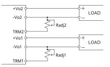
The equations and graphs for the required external resistor (R<sub>adi</sub>) value to obtain a percentage output voltage change of  $\Delta Vo\%$  is as shown in the next page.
