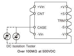
Fig.20-1 Isolation Test
