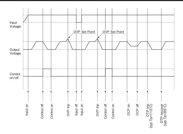
Note: This timing diagram is for negative logic "ON/OFF" option.
