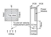
Fig.1-1 Output derating set-up condition
