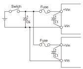
Fig.1-4 Input Filter when Plural Power Modules
