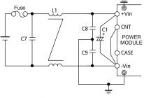
Fig.1-6 Recommended input filter as EMI countermeasure
