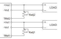
If the external resistor ( $R_{\text{ed}}$ ) is connected between the TRIM pin and –Vo pin, the output voltage will increase. Diagram shown below is the output voltage trim up connection.
