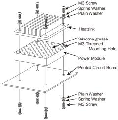
Fig.1-1 Mounting method for standard model
