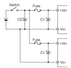
Fig.1-4 Input Filter when Plural Power Modules
