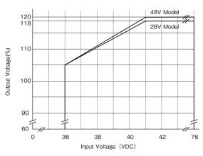
Fig.2-1 Limit of Input Voltage
