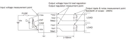
Note: This diagram is for Negative Logic "ON/OFF" Option.
