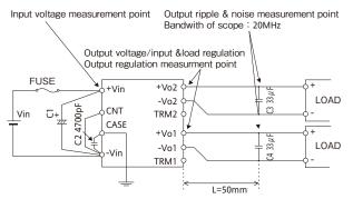
Note: This diagram is for Negative Logic "ON/OFF" Option.
