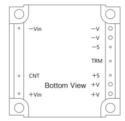
Input and Output Terminal Configurations(Bottom View)
