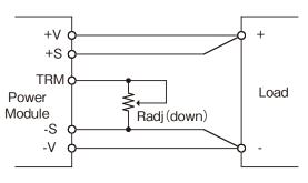
Fig.2-2 Connection for output voltage trim down
