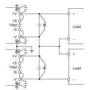
Fig.12-2 Series Operation due to ±Output
