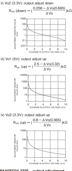
2) PAH75D24-3325 – output adjustment Followings show the equations and graphs for the required
