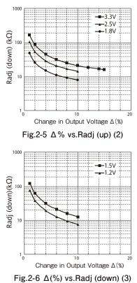
(3) To adjust output voltage for whole range Resistor values, as well as, connecting methods for external resistor (R1) and external variable resistor (VR) are described below.
