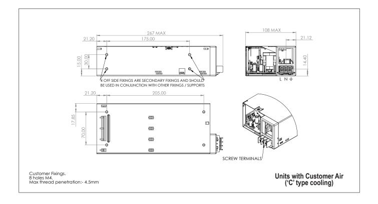
Customer fixings. 8 holes M4. Max thread penetration:- 4.5mm
