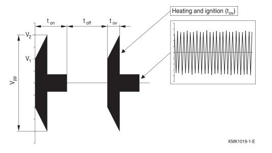
For a repetitive application of on/off switching pulses (as for example in the life tests applied by electronic ballast manufacturers), limits have to be imposed on the time periods under overvoltage and on the duty cycle, in order to keep the capacitance value within the required margins:
