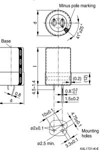
Snap-in terminals, length (6.3 + 1/-1.4) mm. Also available in a shorter version with a length of (4.5 - 1.4) mm.
