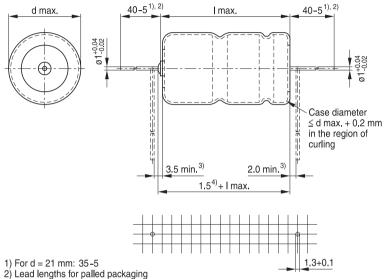
3) Minimum bending distance recommended per wire
