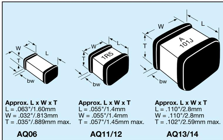
These porcelain and ceramic dielectric multilayer capacitor (MLC) chips are best suited for RF/ Microwave applications typically ranging from 10 MHz to 4.2 GHz. Characteristic is a fine grained, high density, high purity dielectric material impervious to moisture with heavy internal palladium electrodes.
