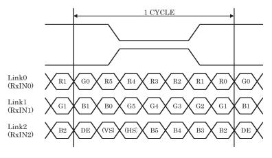
$\begin{array}{l} DE \ : \ DATA \ ENABLE \\ HS \ : \ H_{SYNC} \\ VS \ : \ V_{SYNC} \end{array}$
