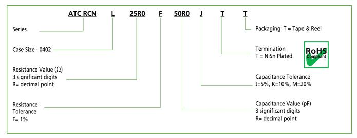
The above part number code refers to an RCN, Case Size L, 25 Ohms, F (1%) resistance tolerance, 50 pF, J (5%) capacitance tolerance, T termination, with tape and reel packaging
