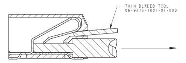
PUSH BLADE (NOT SHARP) INTO SLOT ABOVE WIRE. WHEN WIRE IS FREE, PULL TO EXTRACT.
