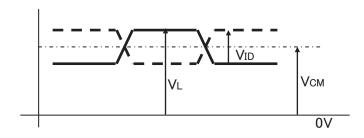
5) V<sub>CM</sub>: LVDS Common mode voltage (V<sub>CM</sub>=1.25V
