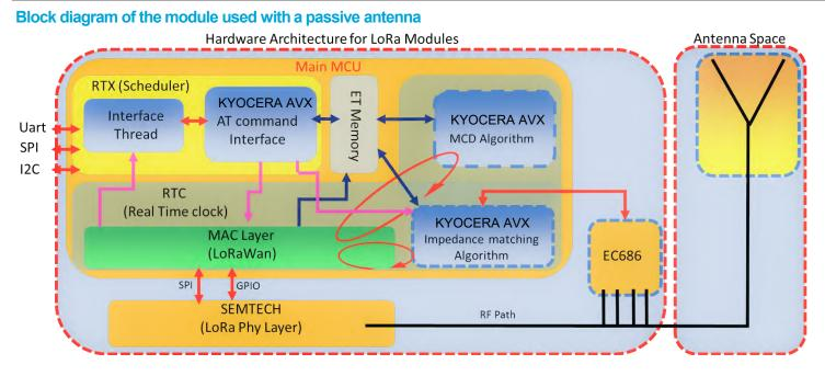
In this configuration, a proprietary impedance matching algorithm helps to maximize the power transfer to the antenna Please refer to the application note about the passive evaluation board for more details [4].
