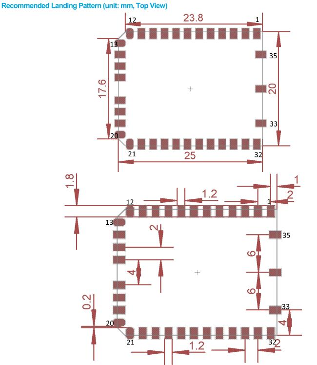
**Note:** Do not place any via or exposed pad in the inner area of the footprint to avoid short circuit between the via on customer board and the via on the bottom side of the EtherLoRa
