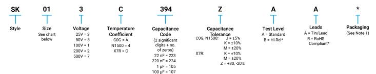
Note 1: No suffix signifies bulk packaging, which is KYOCERA AVX standard packaging. SK01, SK\*3, SK\*4, SK\*5, SK\*6, SK\*9 & SK\*0 are available taped and reel per EIA-468. Use suffix "TR1" if tape & reel is required.
