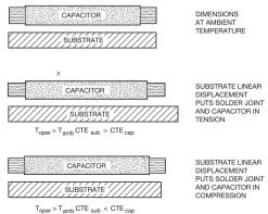
Figure 1. Linear Displacement Between Component and Substrate
