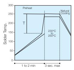
(Preheat chips before soldering) T/maximum 150°C
