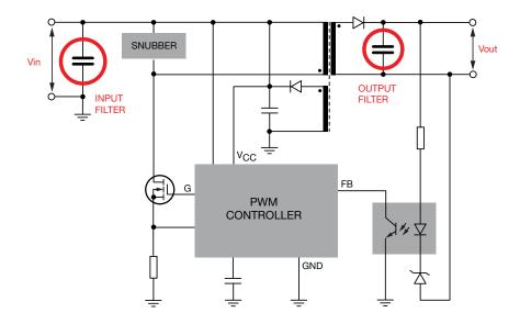
Performance of SMPS capacitors can be simulated by downloading SpiCalci software program http://www.kyocera-avx.com/download/software/SpiCalci-AVX.zip Custom values, ratings and configurations are also available.
