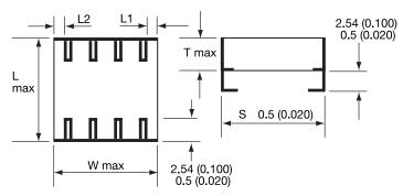
NOTE: A 'J' lead low profile version (CH....0A3) is available with lead height 1.1 (0.043) max. for single chip assemblies eg. CH515C475MA30A3
