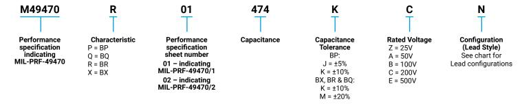
For "T" level parts, replace the "M" in the pin with "T" (for example M49470R01474KCN becomes T49470R01474KCN) PRF-49470 contains additional capacitors that are not available in 87106, such as additional lead configurations and lower profile parts.
