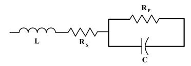
**Reactance** – Since the insulation resistance (Rp) is normally very high, the total impedance of a capacitor is:
