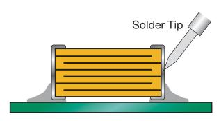
Poor Method - Direct Contact with Part
