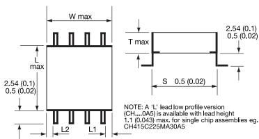
Lead width 0.5 (0.020) Lead thickness 0.254 (0.010)  $L1 = L2 \pm 0.5 (0.020)$
