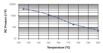
Typical Extended Temperature IR Characterization of VHT/X7R, SMPS Capacitors
