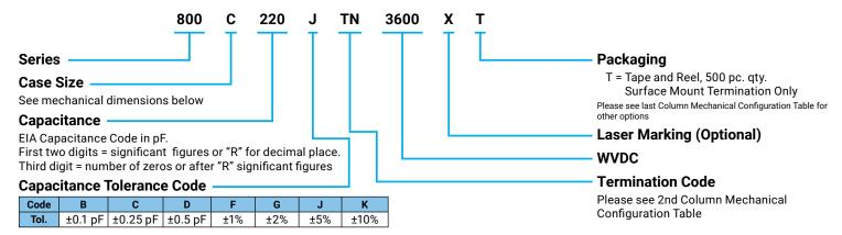
The above part number refers to a 800 C Series (case size C) 22 pF capacitor, J tolerance (±5%),3600 WVDC, with TN termination (RoHS Compliant, Tin Plated over Non-Magnetic Barrier Termination), laser marking and T&R packaging
