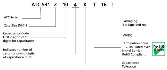
The above part number refers to a 531 Series (case size Z) 100 nF capacitor, K tolerance (±10%), with T termination (tin plated over nickel barrier, RoHS compliant), 16 WVDC, tape and reel packaging.
