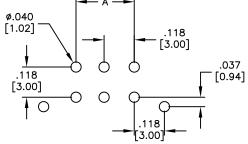
PCB LAYOUT: COMPONENT SIDE RECOMMENDED PCB THICKNESS: .062"[1.57]
