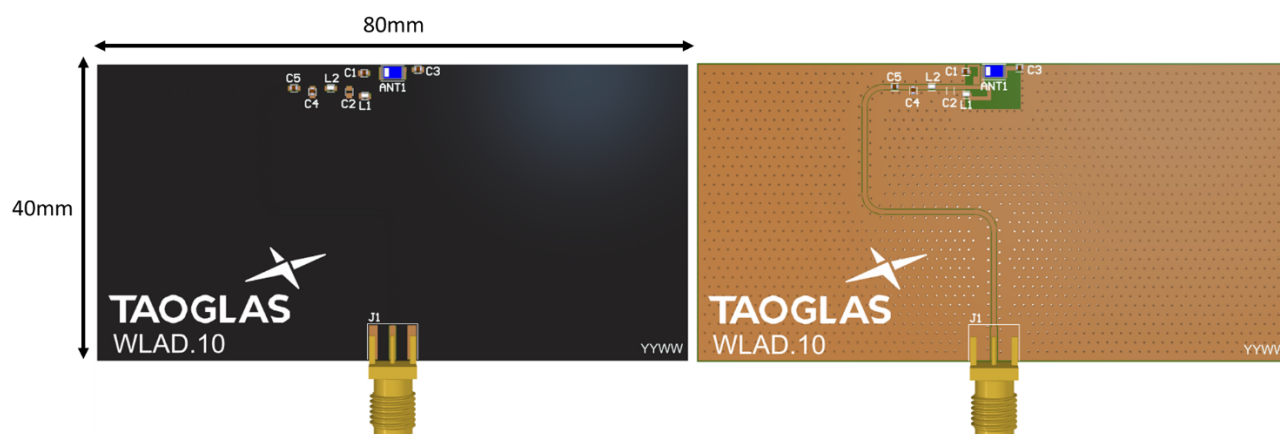
Top Side (WLA.10 placement on 80x40mm PCB)
