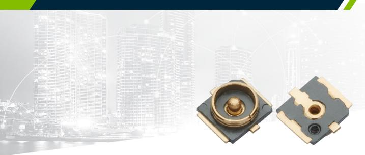
Part of the Taoglas SMD Mount Receptacle, the RECE.20449.001E.01 is a 3-pad type wire-to-board SMD Receptacle solution that is ultra-small, lightweight, and low profile, 1.6mm max. with an operational frequency range of DC to 6 GHz the RECE.20449.001E.01 is gold plated to provide superior performance and allow easy mounting of the male RF connector.
