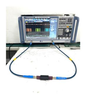
VNA Test Set-up
