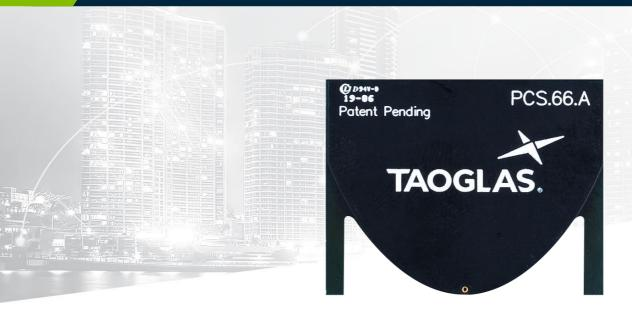
The Taoglas Reach series, are a revolutionary, low profile, small footprint, range of patent pending SMD mount PCB wide-band antennas. The PCS.66.A has been designed to cover all 5G bands, including all sub-6GHz deployments across the 600MHz to 6000MHz spectrum on a very small footprint of just 32 x 25mm. It also covers 3G and 2G bands to allow for fall-back when 5G/4G is not available.
