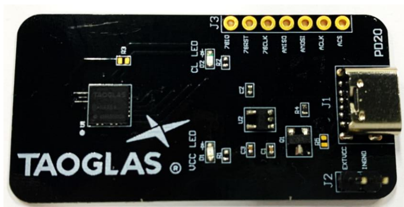
Figure 1 NAA5D.A NFC Evaluation Board
