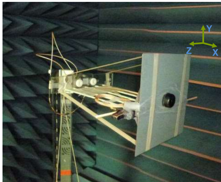
Figure 2. Peak gain, efficiency and radiation pattern measurements.
