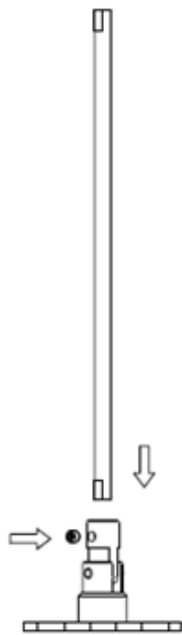
1. Screw locking Torque: 3kgf-cm
