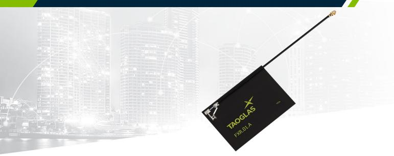
Taoglas has developed an NFC (Near Field Communications) antenna for use with NFC readers. This standard design is matched to a 50 Ohm system and provides a well-matched solution for NFC readers. The antenna is dimensioned to provide the capability of interrogating typical size NFC tags out to a 5 cm. distance. This standard antenna is delivered with a coaxial cable connected to the antenna element to ease use and integration into customer devices.
