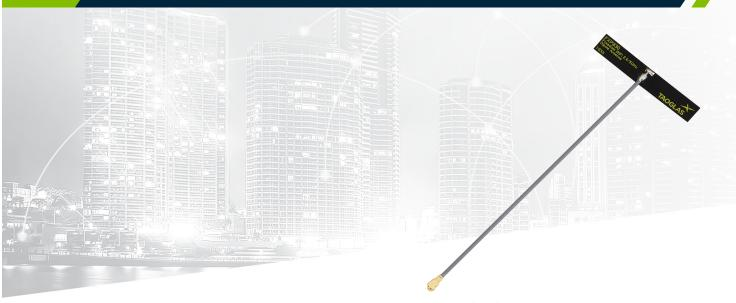
The FXP830 is a high efficiency, small, dipole antenna covering 2.4/5.8/7.1GHz bands including Bluetooth, Wi-Fi and the newly established Wi-Fi 6/Wi-Fi 6E, making this an ideal solution for future-proofing an IoT device. This Taoglas patent pending antenna is unique in the market because it is made from poly-flexible material, has a tiny form factor (42\*7\*.01mm) and has double-sided 3M tape for easy "peel and stick" mounting.
