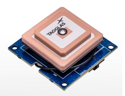
The Taoglas® **EDGE Locate™** solution is an ultra low-power IoT hardware platform providing high precision GNSS for high volume navigation and autonomous applications in an off-the-shelf, compact form factor.
