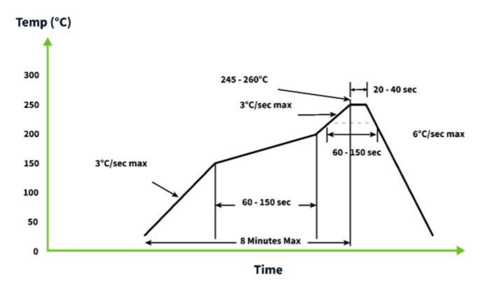
\*Temperatures listed within a tolerance of +/- 10º C
