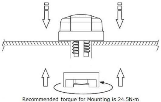
Maximum torque for mounting is 29.4 N·m
