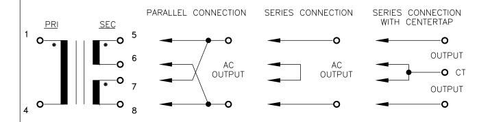
\*not UL-recognized for series connect.
