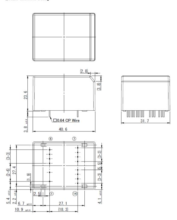
Note :1.The dimensional tolerance without directions is  $\pm$  0.5mm.
