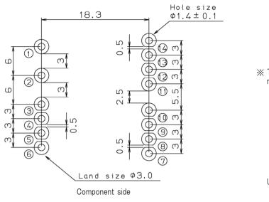
% The round pulling out figure is a pin numbering.
