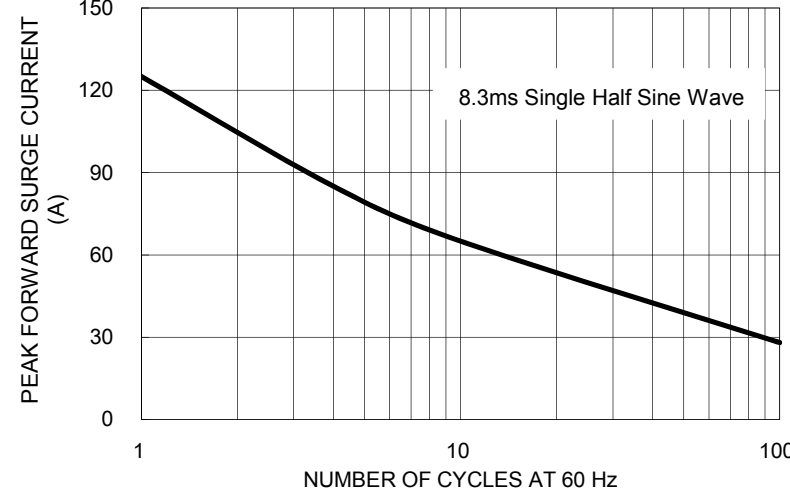
FIG. 3 MAXIMUM NON-REPETITIVE FORWARD SURGE CURRENT
