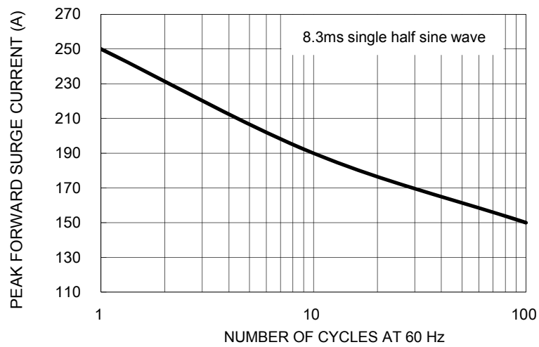
FIG. 7 MAXIMUM NON-REPETITIVE PEAK FORWARD SURGE CURRENT
