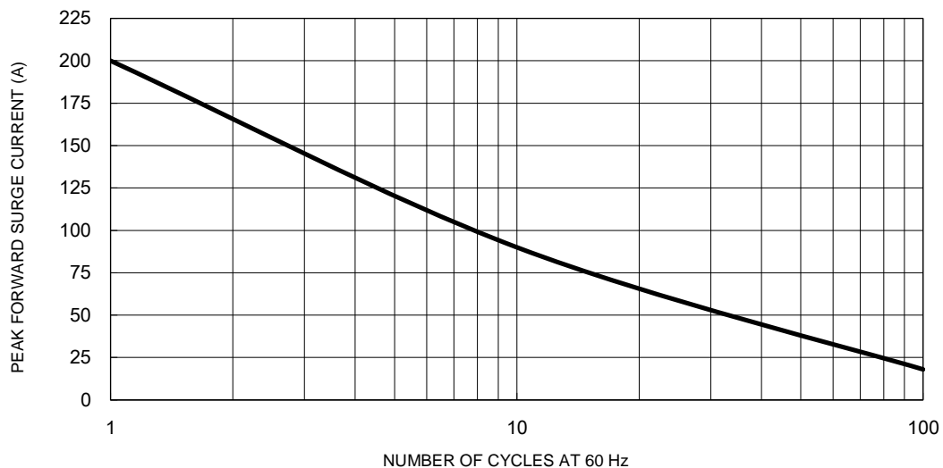
Fig.5 Maximum Non-Repetitive Forward Surge Current
