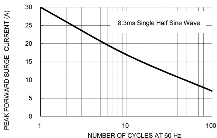
FIG. 3 MAXIMUM NON-REPETITIVE FORWARD SURGE CURRENT
