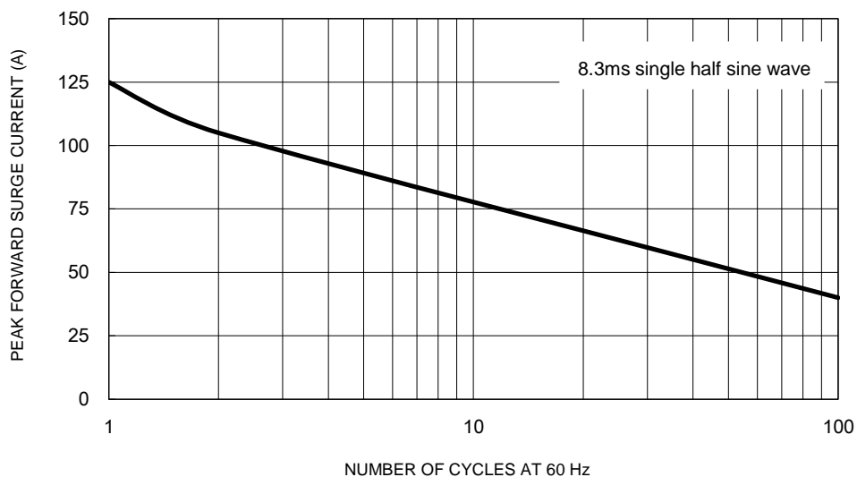
Fig.5 Maximum Non-Repetitive Forward Surge Current
